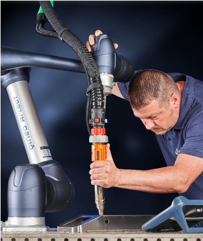
Photo 3: The QINEO ArcBoT relieves employees and ensures consistent, reproducible welding quality.
