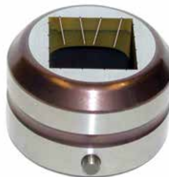
Photo 1: Mate Slug Free Light notches are cut at an angle to create a series of protrusions on the slug. As the slug moves through the die, the protrusions become trapped against the die land to prevent the slug pulling back on to the sheet. (Image enhanced for additional clarity)
